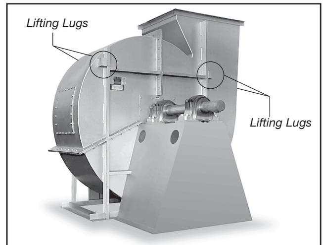
Housing should be lifted using straps and spreaders. Do not distort housing or side plates when lifting.
