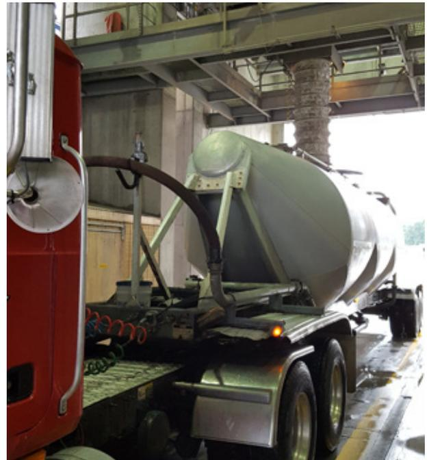
positioning establishes an optimal material flow pattern through the spout, minimizes wear, and creates favorable spout life cycle costs. Additionally, the combination of the spout's telescoping and positioning ability creates labor savings costs in not having to hire employees to perform these tasks.
