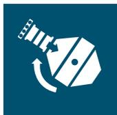
3) Valve automatically opens at approximately 110° as unit rotates at 1.5 rpm.
