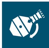
4) Drum empties completely, valve automatically closes at approximately 240° and unit continues to 0° position.
