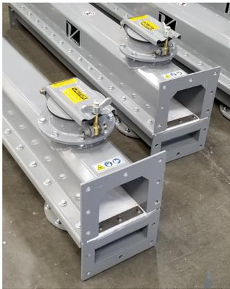
An air-gravity conveyor is a device for moving dry, light-weight, easily fluidized powders. The conveyor consists of a rectangular chamber separated by an air-permeable, porous media material. The media creates two separate chambers within the conveyor: A top chamber to handle the product to be conveyed, and a bottom chamber to handle compressed air.
